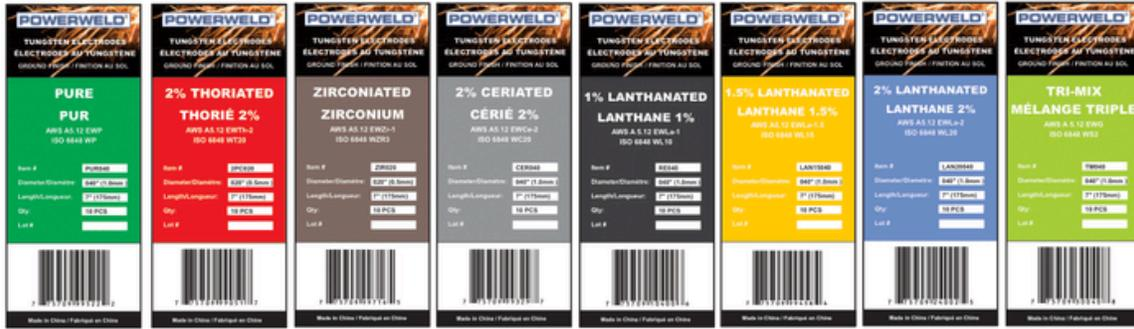
PowerWeld offers eight types of tungsten electrode to cover every TIG welding application. Electrodes are 7" (175mm) in length and packaged 10 rods per box. All tungstens have color coded tips for easy identification, and meet AWS A5.12 specifications. Electrodes are supplied with a smooth, round, bright centerless ground finish.
