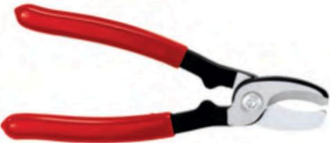
Cable Cutter, Shear Cut, Overall Length 9-1/4 In., Handle Design Dipped, Features High Leverage Design for Superior Cutting Ability, Designed with a Shear-Type Jaw for Cutting Aluminum and Soft Copper (Not for Use on Steel or ACSR type Cables), Cuts up to 100-Pair Cables, Made of Chrome Vanadium Steel
