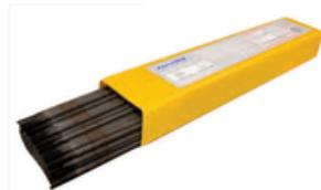
**PowerWeld 7018** is a low-hydrogen electrode for use in all positions on low, medium and high-carbon steels. 70,000 PSI tensile strength. Ideal for out of position welding and tacking. Runs on AC or DCEP (reverse) polarity. Features a steady arc with low spatter and medium penetration, providing X-ray quality weld deposits.
